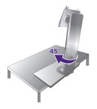
Tighten the thumbscrew on the bottom of the monitor base as illustrated. And then turn the stand counterclockwise to face forward.
