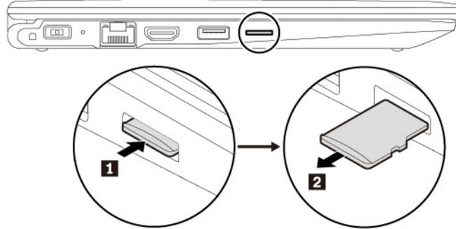
3. Insert the new card into the microSD card slot. The card might stop before it is installed into the card reader. Ensure that you insert the card firmly until you hear a click.
