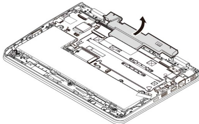
7. Install the new speaker assembly in place.
