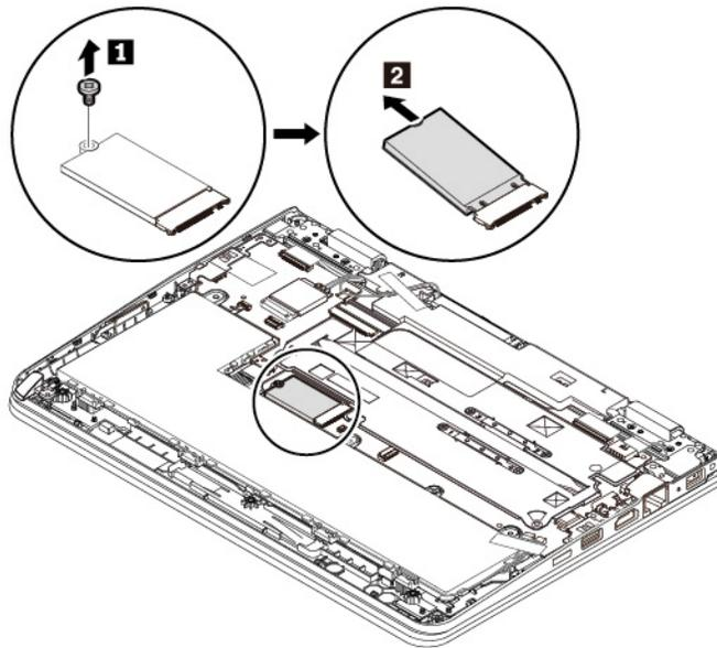
6. Insert the new M.2 solid-state drive into the slot at an angle of about 20 degrees **1**. Pivot the M.2 solid-state drive downward **2**. Install the screw to secure the M.2 solid-state drive **3**.
