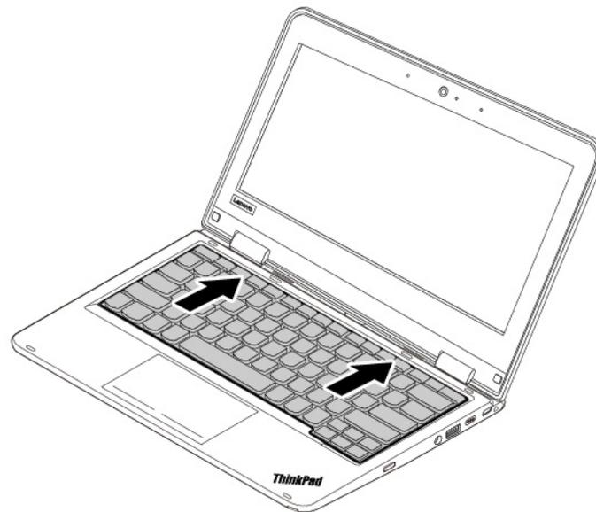
7. Lift the keyboard slightly as shown **1**. Pivot the keyboard slightly upward to remove it **2** from the keyboard bezel.
