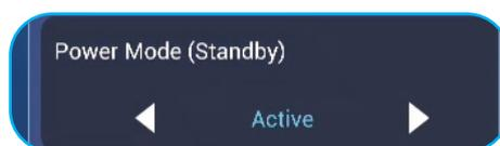
**Note:** *Optoma ProService and LAN control remote power on functions will only work when Power Mode (Standby) is set to Active.*
