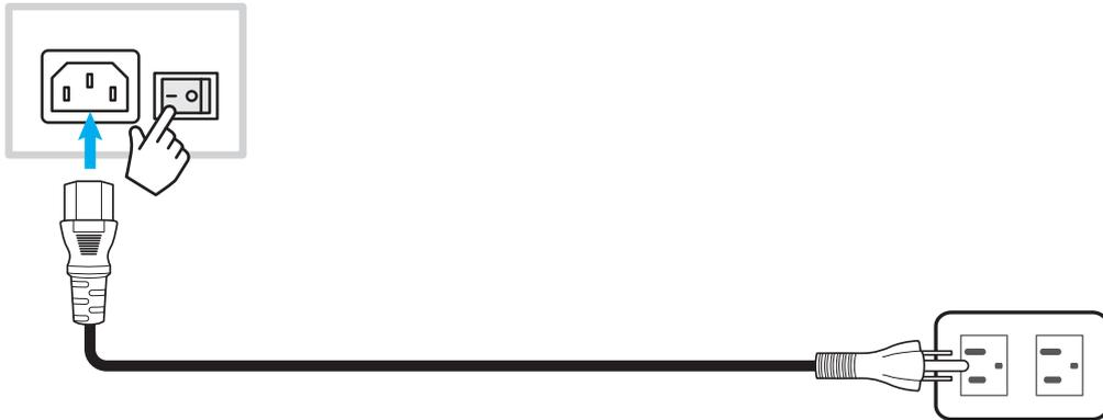
Press the **Power** button to turn on the IFP. The LED indicator light turns white, indicating it is ready to use.
