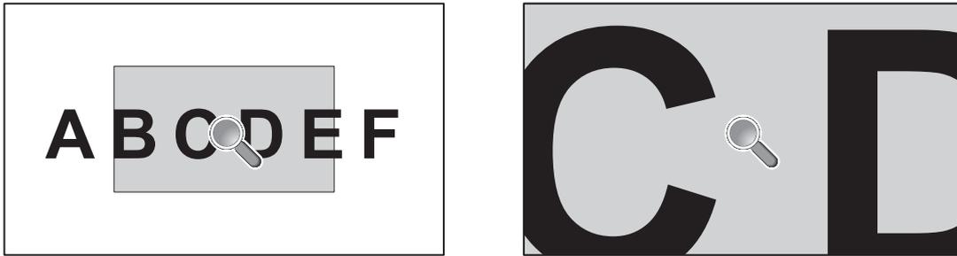
The [POINT ZOOM] function increases the image size and expands it horizontally and vertically simultaneously. The image can be increased up to 10 times its size.
