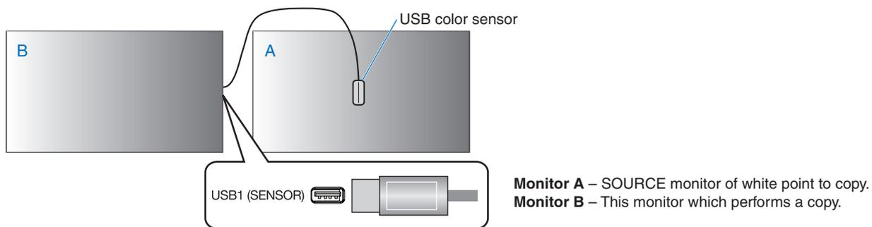
**NOTE:** When adjusting the color of multiple displays, we recommend that you perform [SELF CALIBRATION] from [WHITE COPY].
