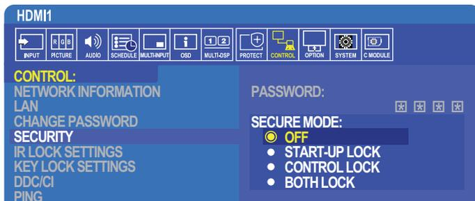
1. Using the remote control navigate to [CONTROL] then to [SECURITY].
