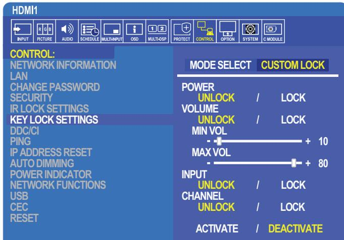
1. Using the remote control navigate to [CONTROL] then to [KEY LOCK SETTINGS].
