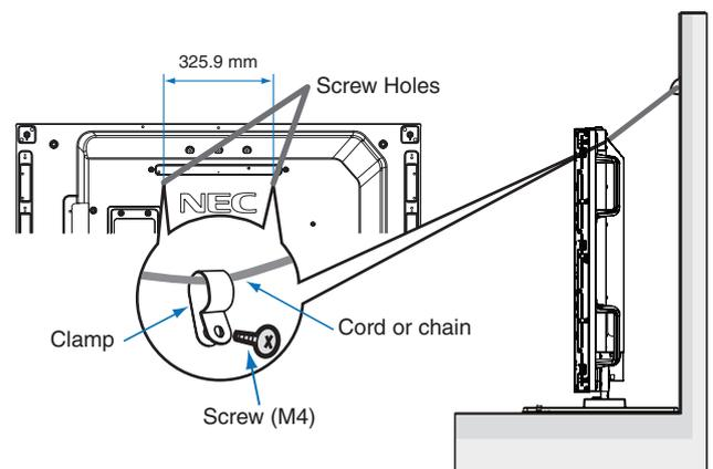
Before attaching the monitor to the wall, make sure that the wall can support the weight of the monitor.
