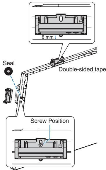
**Fixed by screw:** Remove the seal covering screw holes on the bezel. Secure the unit with the attached screw. Set the sensor unit close to the back side.
