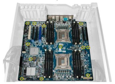
5. Lift the system board in an upward direction and remove it from the computer.
