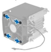
4. Remove the heat-sink fan from the heat sink assembly.
