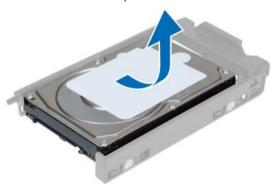
9. If a 2.5 inch hard drive is installed, Push the retention clips in an outward direction and lift up the drive to remove it from the 3.5 inch hard-drive caddy.
