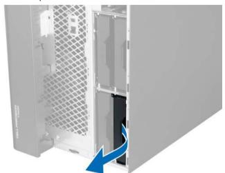
4. Slide the hard-drive bracket in an outward direction to remove it from the computer.
