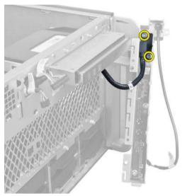
8. Remove the screws that secure the I/O panel and remove it from the computer.
