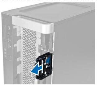
7. Flex the hard-drive bracket on both sides to loosen the hard drive.
