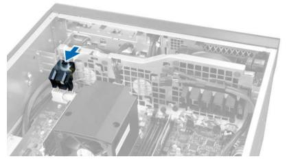
5. Lift the air duct in an upward direction to remove it from the computer.
