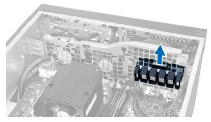
9. Route the system-fan cable through the opening in the system-fan module.
