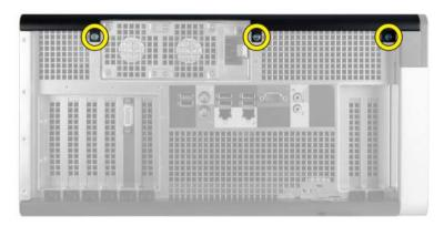
3. Slide the right cover in the direction indicated to remove it from the computer.
