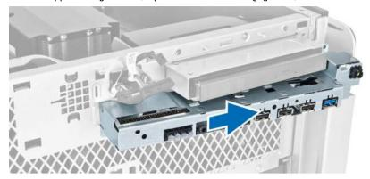
7. Remove the screws that secure the USB 3.0 module to the I/O panel and remove it from the computer.
