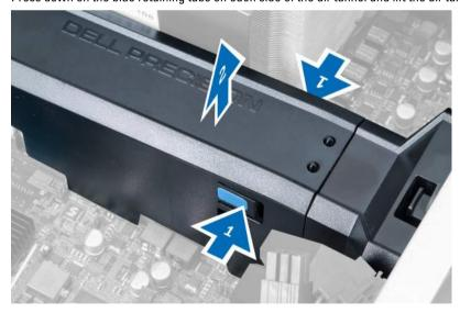
4. Press down on the release latch on the other side of the air tunnel module to release it from the chassis.
