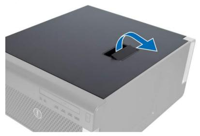
3. Lift the cover upward to a 45-degree angle and remove it from the computer.
