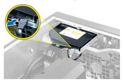
5. Press down on the blue release tab to release the latches that secure the optical drive.
