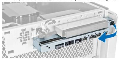
6. Slide the opposite edge of the I/O panel outward to disengage the I/O module from the chassis.
