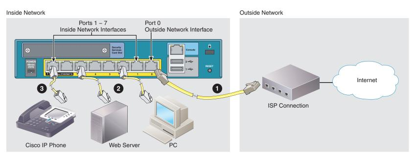
If you connect a server (such as a web server) to the ASA, you can use ASDM to make services on that server accessible by internal and external users. See "7. (Optional) Allowing Access to Public Servers Behind the ASA."
