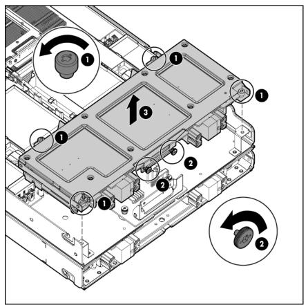
To install the interposer board, reverse the removal procedure.
