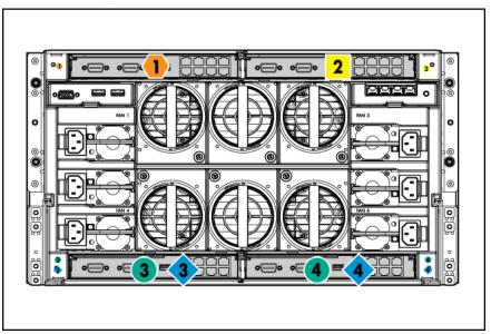
To support network connections for specific signals, install an interconnect module in the bay corresponding to the embedded adapter or mezzanine signals.
