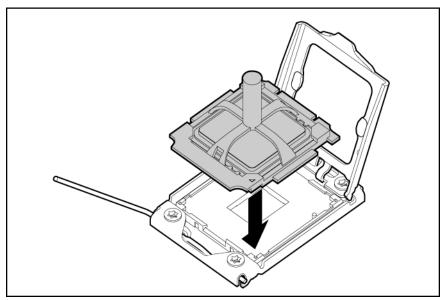
**13.** Press down firmly until the processor installation tool clicks and separates from the processor, and then remove the processor installation tool.
