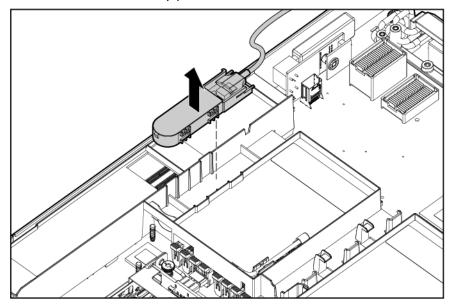
• Remove the battery pack from the right DIMM baffle.
