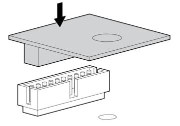
6. Install the TPM security rivet by pressing the rivet firmly into the system board.
