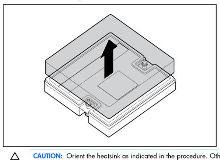
**CAUTION:** Orient the heatsink as indicated in the procedure. Otherwise, you cannot install the hard drive cage.
