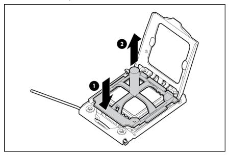
14. Close the processor socket retaining bracket and the processor retaining latch.
