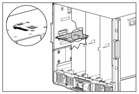
2. Push the device bay shelf back until it stops, lift the right side slightly to disengage the two tabs from the divider wall, and then rotate the right edge downward (clockwise).
