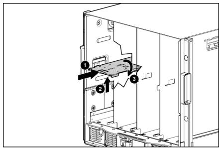
3. Lift the left side of the device bay shelf to disengage the three tabs from the divider wall, and then remove it from the enclosure.
