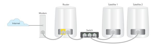
Figure 6. Ethernet backhaul connection using a switch
