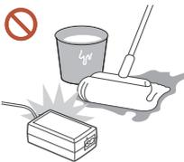
**Do not let water enter the AC/DC adapter device or get the device wet.**
