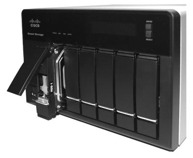
**STEP 7** Using your thumb, apply even pressure to the middle of the tray while you insert the tray slowly and fully into position in the chassis.
