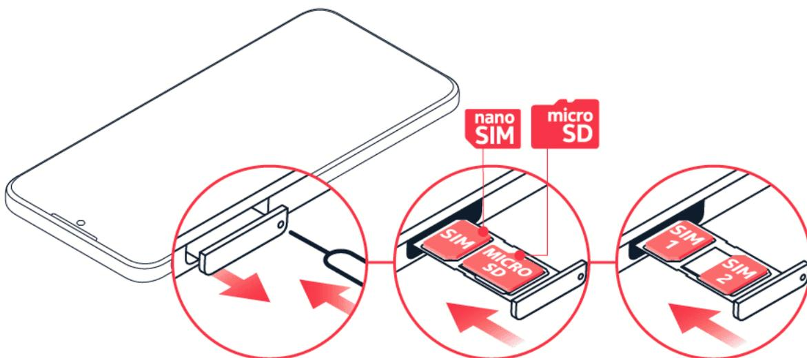
1. Open the SIM and memory card tray: push the tray opener pin into the tray hole and slide the tray out.
