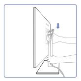
Hold the bottom of the stand bar Installation is finished. securely with left hand, steadily hold the top of the stand bar with right hand, then use the thumb of right hand to press and push the cover stand rear downward.
