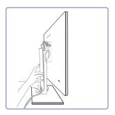
Hold the cover stand rear with right hand, and fix the cable into the groove in the cover stand rear with left hand.
