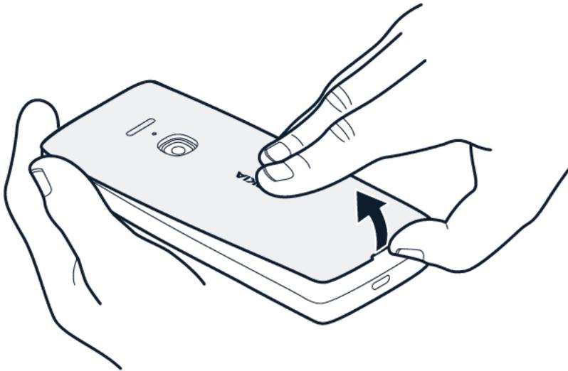
1. Put your fingernail in the small slot at the top of the phone, then lift and remove the cover.
